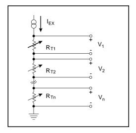
Figure 8. RTD Measurement with SCXI-1122
