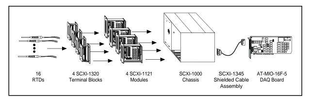
Figure 5. SCXI System for Monitoring 16 RTDs
