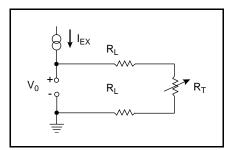
Figure 2. Two-Wire RTD Measurement
