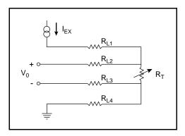
Figure 3. Four-Wire RTD Measurement
