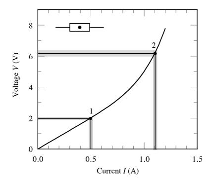
Figure 7.1 V-I curve for a nonlinear resistance
