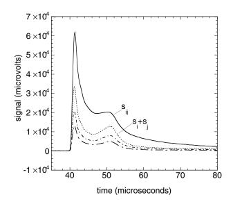
FIG. 1. This shows the bolometer signals for the two separate pulses (dash-dotted lines) and for the double pulse (solid line). The sharp peak at 41  $\mu$ s is due to the l phonons; the signal after  $\approx$ 44  $\mu$ s is due to the h phonons. The sum of the signals from the two separate pulses is shown as the dotted line; it can be seen to be about half that of the double pulse. The input pulses are 100 ns and 6.3 mW.
